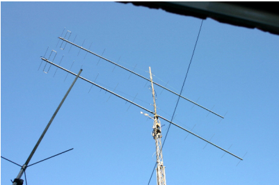
2 x 14el InnovAntennas LFA Yagis installed at G4KWQ
