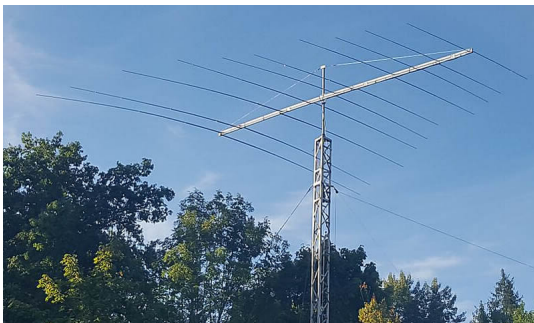
The Twin-boom feedline of the BOLPA-10 can easily be seen in this image
