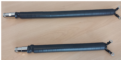
Examples of the InnovAntennas ferrite core baluns
