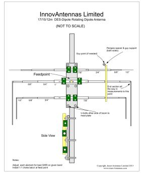
The DES-dipole Antenna Layout
