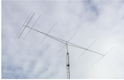
A 7 element OWL Super-Light 50MHz / 6m DX Yagi / low noise Yagi
