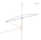
The above shows the current (represented by the pink line) distribution through the driven element of a correctly balanced Yagi with a balun at the feed point.
