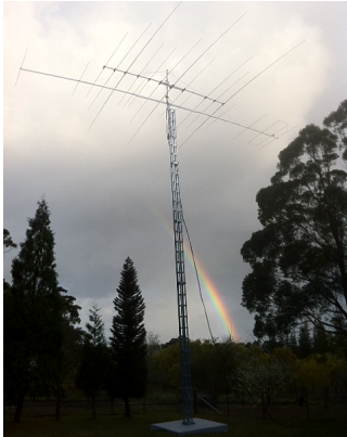
The 8el 50MHz InnovAntennas LFA at VK2IZI
