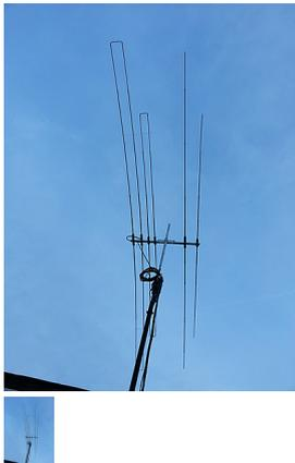
A super-compact dualband 7/10MHz WARC band Yagi with single feedpoint
