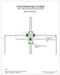
The DES-dipole Antenna Layout
