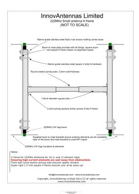
An H frame for 4 x 14el 222MHz LFA Yagis
