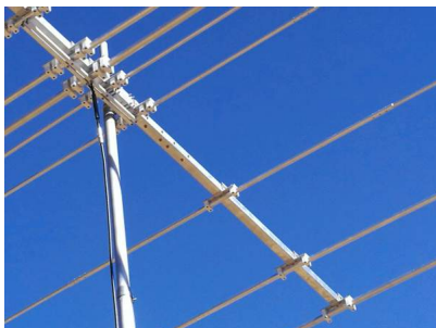
View of the 50mm (2") Square boom and element holders on the rear of the antenna
