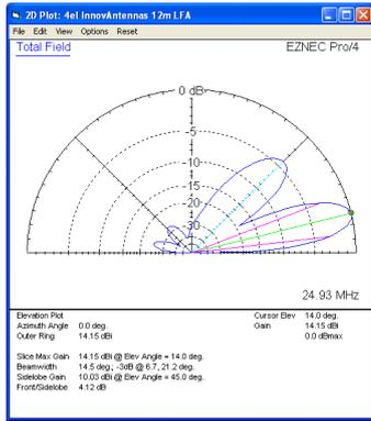
Single 4 element LFA up 12m above ground
