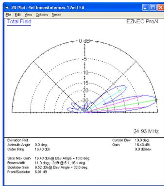
2 x 4 el LFA Yagi 6.6m apart with the bottom antenna 12m above ground
