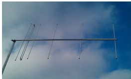
A 6 element OWL (Optimised Wideband Low Impedance) Super-Light Yagi for 144-148MHz
