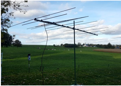
The 12el Duo @ ON8ID before installation on the tower
