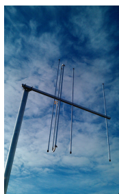
Custom Marine Band (155MHz - 157MHz) OWL Yagi -
