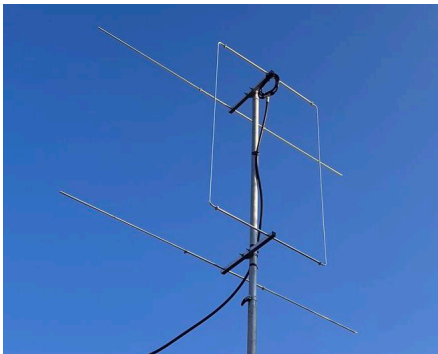
The 3el Slot-Q on test with the provided coaxial 'Loop' Balun. rear mounted version shown, centre mounted version also available.
