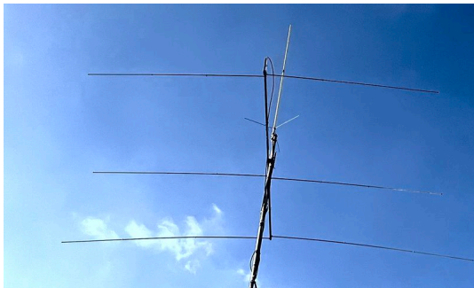
The BOLPA-3 on a tiny 3.6m boom installed and ready to go
