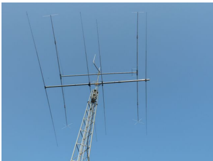
The Delta C-240 above a 20m 4el Yagi for size comparison
