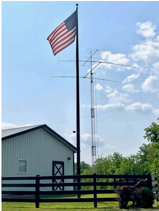
The Delta C-240 below a 50MHz 6el LFA Yagi at K9US
