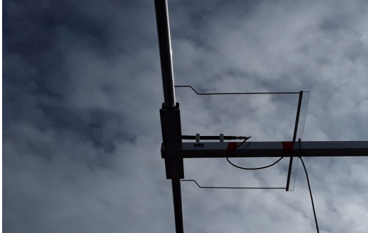
The Large diameter Hairpin of the Delta C-240 that contributes to the exceptional bandwidth of this antenna
