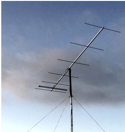
A 7el 144MHz OWL Ultra installed and ready for action
