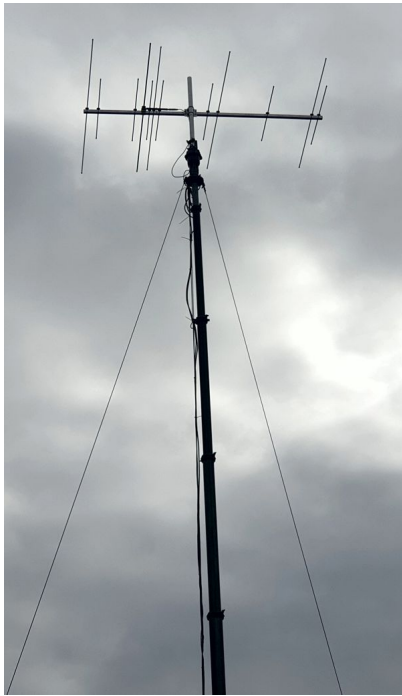
The 12el Duo installed at M0VOZ
