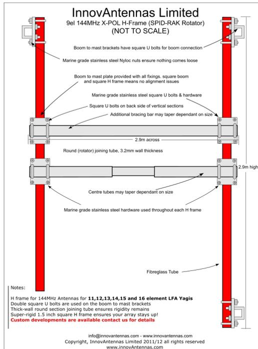
An H frame for 4 x 9el X-POL 144MHz LFA Yagis
