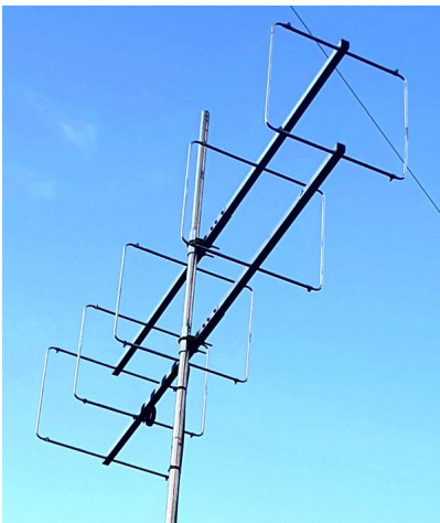
The 5el LFA-Q Long Boom installed at G0EIG
