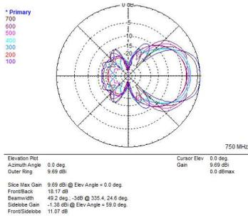
**Pattern overlay between 100MHz and 750MHz showing good F/B throughout**
