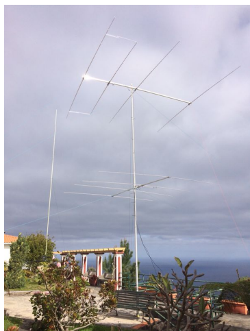
The 4el 21Mhz OP-DES Yagi /P (top) in Maderia Island (UA9CDC)
