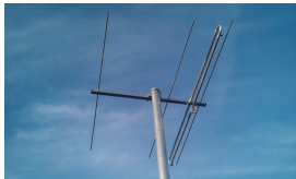
A 4 element OWL (Optimised Wideband Low Impedance) Super-Light Yagi for 144-146MHz
