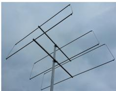
**A 3 element LFA-Q (Super-rigid Quad-style) Super-Light Quad Style Yagi for 50-50.5MHz**
