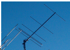
2.5 A 5 element OWL (Optimised Wideband Low Impedance) Super-Light Yagi for 69.9-70.5MHz
