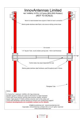
An H frame for 4 x 4el X-POL 144MHz LFA Yagis
