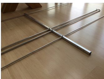
The super-light OWL's have elements connected and through the boom with a single securing bolt (3el rear mount OWL featured
