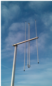
A 3 element OWL (Optimised Wideband Low Impedance) Super-Light Yagi for 50.0 - 50.4MHz
