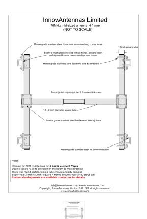
An H frame for 4 x 5el 70MHz LFA Yagis
