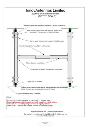
An H frame for 4 x 12el 222MHz LFA Yagis
