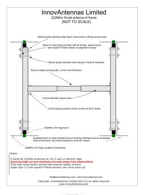
An H frame for 4 x 11el 222MHz LFA Yagis
