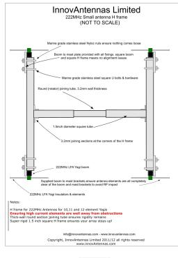
An H frame for 4 x 10el 222MHz LFA Yagis
