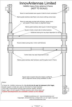
An H frame for 4 x 13el 144MHz LFA Yagis
