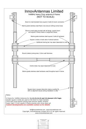
An H frame for 4 x 12el 144MHz LFA Yagis
