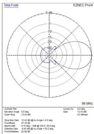
A Broadband OP-DES Yagi for 88 - 108MHz - 20 element
