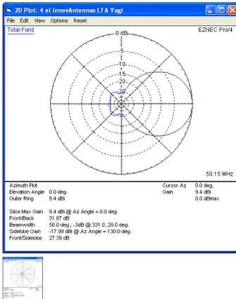
A Very low-noise 50MHz LFA Yagi
