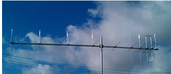
A single 18el (9+9) X-pol LFA Yagi
