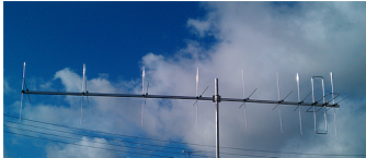
A single 18el (9+9) Xpol LFA Yagi
