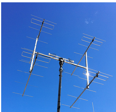
EME in a box! 4 x 6el InnovAntennas LFA Yagis on test as a small EME Array
