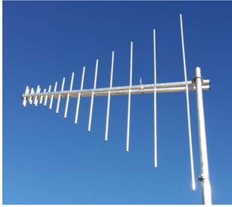
A short-boom, high quality Log Periodic Dipole Array for 100MHz to 750MHz
