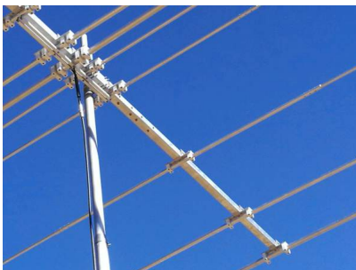
View of the 50mm (2") Square boom and element holders on the rear of the antenna
