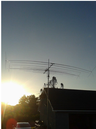
A European version of the XR6C (Compact) installed at GI0TSS (MKII with capacity loading, not yet available)
