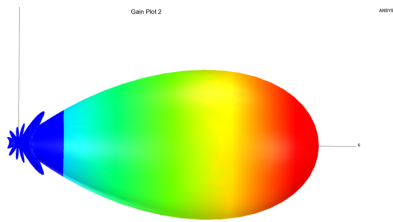
Elevation Plot of the 9el OWL Ultra presented within Ansys HFSS
