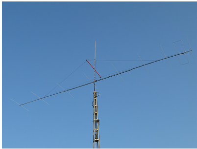
An InnovAntennas 9el LFA Yagi installed at EA7KW
