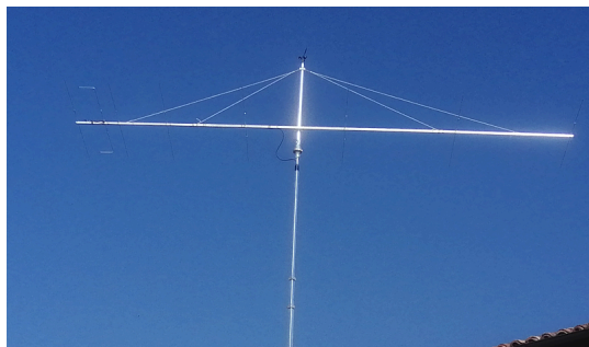
A single 8el 50MHz OP-DES @ I2HBW
