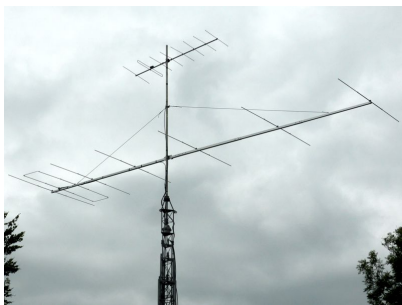
The 7el WOS installed are G2SJX
