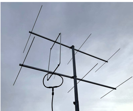
The 7el Slot-Q on test with the provided coaxial 'Loop' Balun. rear mounted version shown, centre mounted version also available.
