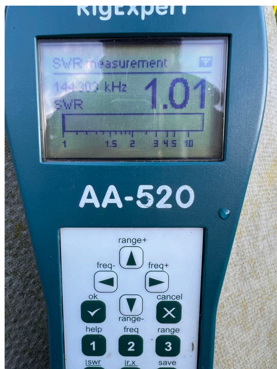
Measured SWR @ 144.300MHz
