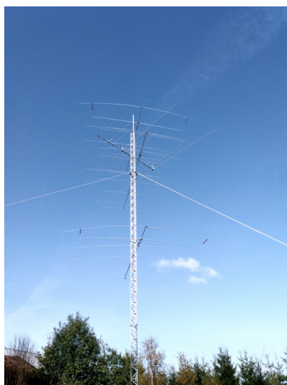
2 x 5el OP-DES Stack for 20m at OH6MW
