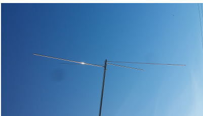
A close-up of the Capacity loaded end sections of the Delta 2-140 and the 'spiral' configuration of the spokes which are 8mm diameter
